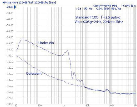
and then observing the effect on the output spectrum. When the applied vibration is a single frequency sine wave, a discrete spur will be produced offset from the carrier by the vibration frequency. By measuring the level of this spur relative to the power of the carrier, the amount of frequency devi-
